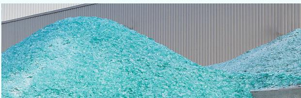
Gerresheimer has worked intensively to reduce the proportion of raw materials used in clear glass (sand, calcium oxide, and sodium carbonate) to just 45% of the batch melted in the furnace. The composition of this glass has been tested and certified by RDC Environment of Belgium.
