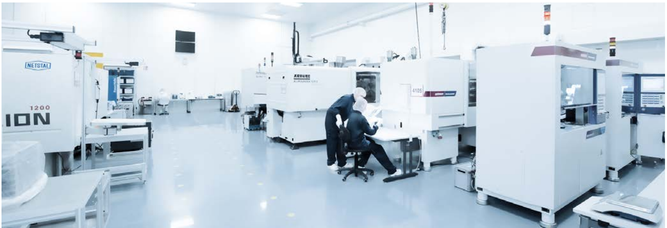
Our small batch production in class 8 cleanroom in accordance with DIN EN ISO 14644-1 in Wackersdorf, Germany
