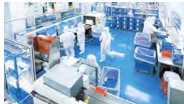
Injection molding and assembly of inhaler in the ISO 14644-1 ISO class 8 clean room in Dongguan City, China
