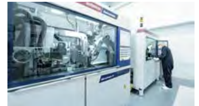
Micro injection molding system in a clean room in accordance with ISO 14644-1 ISO class 8
