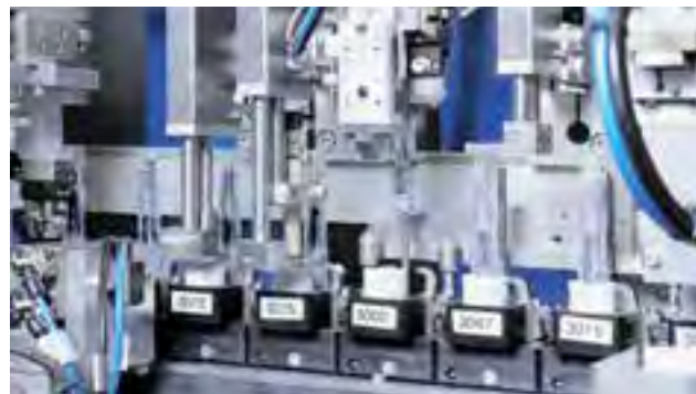
Fully automatic insertion of a spring into an autoinjector in the clean room according to ISO 14644-1 ISO class 8 in Pfreimd, Germany
