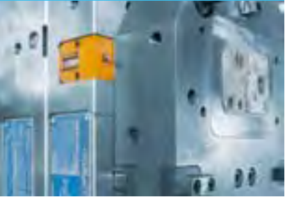
Two-cavity mold for a laboratory disposable
