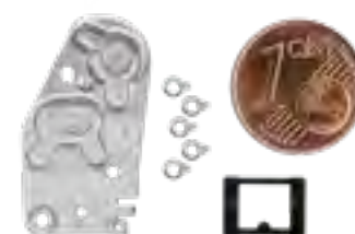
Micro injection molded parts of an infusion pump
