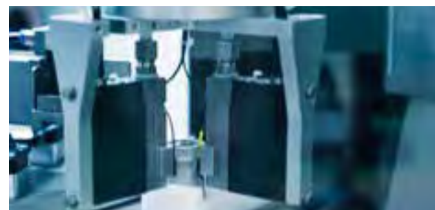
Vaseline metering to improve gliding properties
