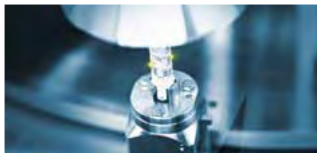
Laser marking of a plastic part for an insulin pen
