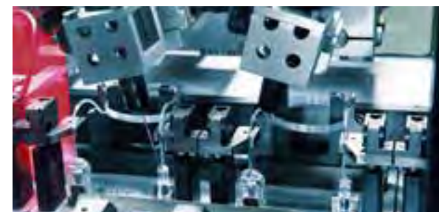
Gluing of tube and coupling part with subsequent flow inspection
