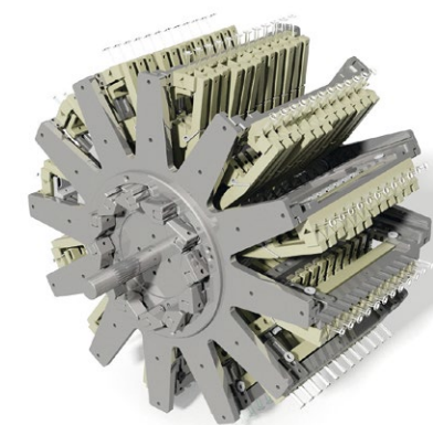
The drum of a washing machine for the cleaning of syringes in order to reduce glass and tungsten residuals
